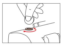
The presser foot pressure has been preset at the factory and rarely needs adjustment. You may find it necessary, however, to decrease the pressure for thick fabrics or increase pressure for thin fabrics to feed more smoothly under the presser foot. Use a coin to turn the screw on top of the machine.
