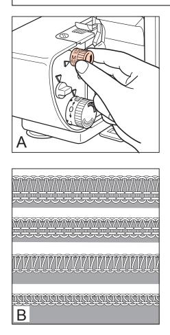
The stitch width adjusting dial is located above the stitch length dial (fig. A). The stitch width dial displays two sets of numbers, indicating two width ranges. The larger size numbers on the dial, 5.5 through 7.5mm, denotes the stitch width dial when the left needle is in use. The smaller size numbers, 3.0 through 5.0mm, apply when the right needle is in use.
