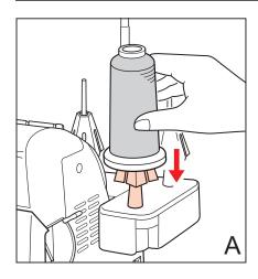
When using threads on cones or king spools, place the cone or spool securely over the cone holders furnished on your machine. To avoid bending the thread stand, you may need to place one hand under the stand while positioning the cone. The cone holders prevent the cone or spool from spinning, enabling the thread to feed evenly (fig. A).
