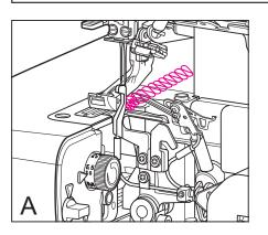
As you sew, you will discover that maneuvering the fabric is different from conventional sewing because the threads form around the stitch fingers (fig. A).
