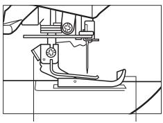
Presser Foot Release Button Seam Line Guides This serger has the convenience of a snap-on presser foot.
