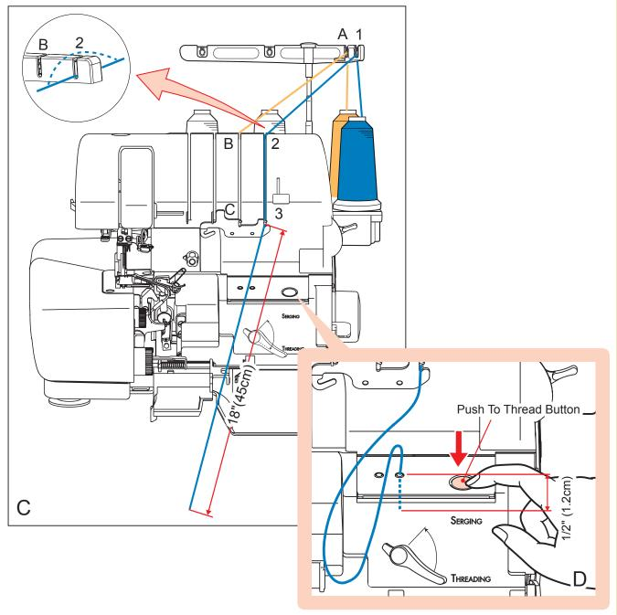
\*Be sure at least 1/2" of thread is inserted into the threading port.
