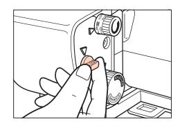
When no trimming is desired, as when stitching on a fold, flip the cutting blade lock switch clockwise to the LOCK position. The cutting blade no longer moves up and down, but remains in its lowered position. To re-engage the cutting blade, turn the cutting blade lock switch half of a turn counter-clockwise. The blade will start moving automatically when you start sewing.
